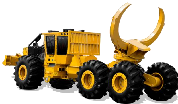
Slika 8. Tigercat C640H - klam bank skider ( www.tigercat.com/product/c640h-clambunk-skidder/ )
